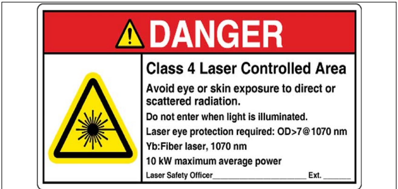
Figure 1. A sample laser warning sign including the international symbol for laser radiation
