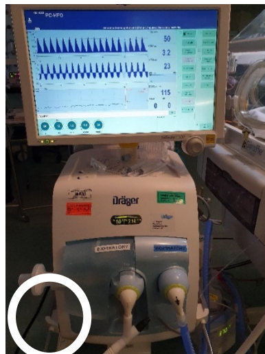
Figure 1. Draeger VN500 ventilator. An external viral filter can be connected to the exhaust hose (circled).
