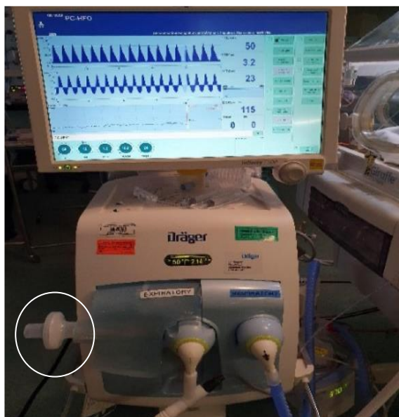
Figure 1. Draeger VN500 ventilator. An external viral filter can be connected to the exhaust hose (circled).
